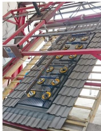
Wind uplift pressures are higher when solar is roof integrated and the wind resistance of some integration products is not high enough even for low-rise scenarios (see chart).
